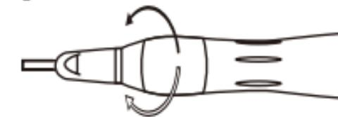
Excessive loads generated by defective burs rotating at 40,000 rpm will quickly damage the ball bearings.
